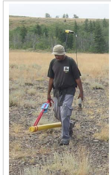
Figure 10. Field mapping ground conductivity using a Dualem EMI sensor at the USDA - Reynolds Creek experimental watershed in Idaho.
