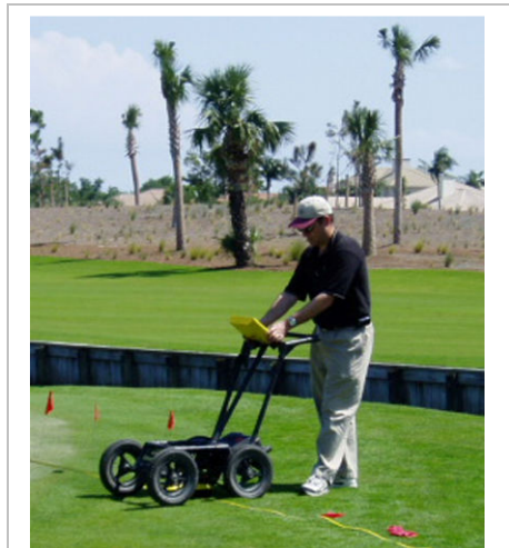
Figure 12. Noggin smart cart GPR, courtesy of Sensors and Software inc.
