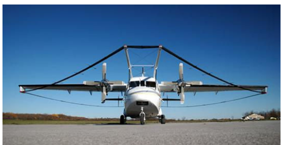
Figure 4. The GEOTEM time-domain fixed-wing EM system.
